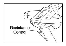
to decrease the resistance, turn the control counterclockwise. Important: Stop turning the control when rotation becomes difficult or damage may result.
